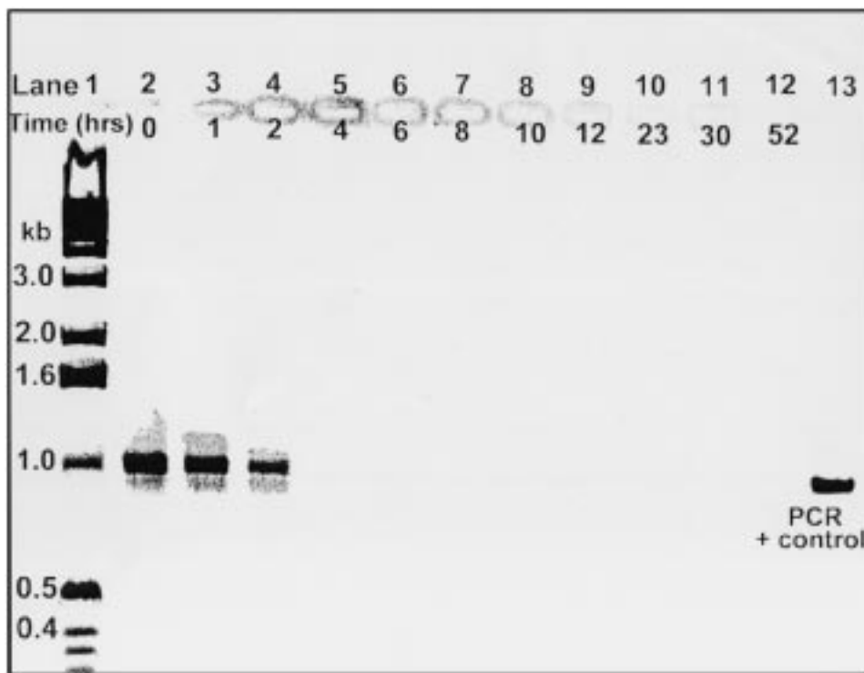
Figure 1 Enhanced contrast image of agarose gel containing pBR322 DNA PCR products extracted at various time intervals from a wastewater-derived matrix. Lane 1: molecular weight markers; lanes 2–12: extracted PCR-amplified 1.04-kb pBR322 DNA PCR products after varied exposures to wastewater as shown below lane numbers; lane 13: amplified positive control, amplified fragment from pBR322 in TE buffer.
